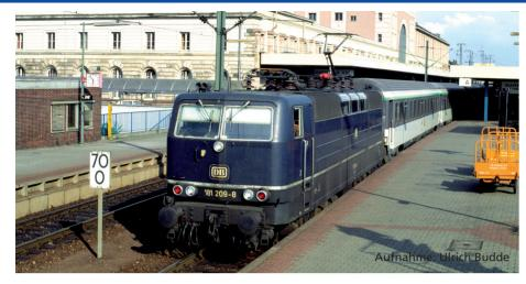
In 1972, the Deutsche Bundesbahn ordered dual-frequency locomotives under the designation 181.2 for traffic to France and Luxembourg. According to its The 25 locomotives were delivered on cross-border routes at speeds of up to 160 km/h in express service, including in front of the famous Orient-Express.
